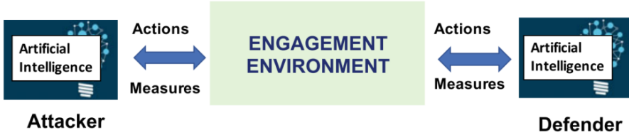
Fig. 1 Overview of coevolutionary adversarial AI framework concept. The coevolutionary component performs search over the actions of adversary controllers. The engagement component evaluates the strategies of the adversaries and returns the measurements of the engagement
