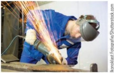
Figure 4.12 Energy Consumption Electrical energy is consumed as the motor of the grinder does work and turns the grinding wheel. Notice the flying sparks and that the operator wisely is wearing a face shield. An electric power company is actually charging for energy in units of kilowatt-hours (kWh).
