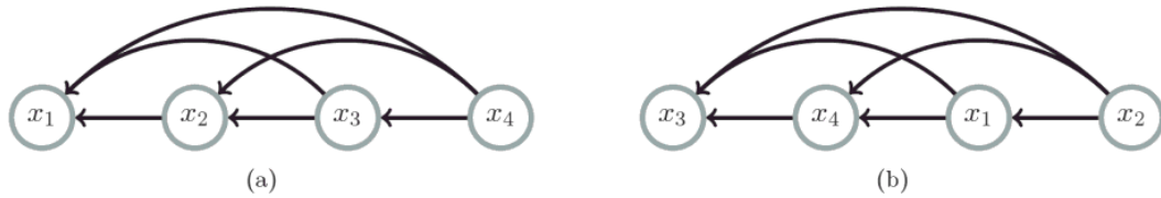
Figure 3.4 Two BNs for a four-variable distribution. Both graphs (a) and (b) represent the same distribution p(x_1, x_2, x_3, x_4) . Strictly speaking they represent the same (lack of) independence assumptions – the graphs say nothing about the content of the tables. The extension of this ‘cascade’ to many variables is clear and always results in a directed acyclic graph.
