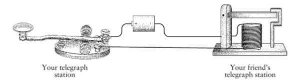
As we discovered, you don't need two wires connecting the two telegraph stations. One wire will suffice if the earth provides the other half of the circuit.
