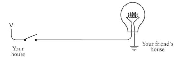
The V stands for *voltage*, but it could also stand for *vacuum*. Think of the V as an electron vacuum and think of the ground as an ocean of electrons. The electron vacuum pulls the electrons from the earth through the circuit, doing work along the way (such as lighting a lightbulb).
