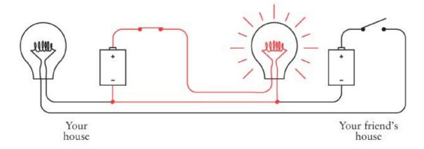
No electricity flows in the other part of the circuit because there's no place for the electrons to go to complete a circuit.
