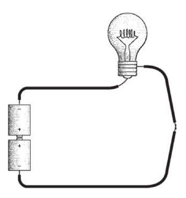
The two positive ends of the battery need electrons for the chemical reactions, but there's no way electrons can get to them because they're attached to each other. If the two positive ends of the battery are connected, the two negative ends should be also:
