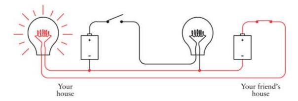
When you and your friend both try to send at the same time, sometimes both switches are open, sometimes one switch is closed but the other is open, and sometimes both switches are depressed. In that case, the flow of electricity in the circuit looks like this:
