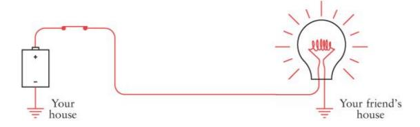
The electrons come out of the earth at your friend's house, go through the lightbulb and wire, the switch at your house, and then go into the positive terminal of the battery. Electrons from the negative terminal of the battery go into the earth.
