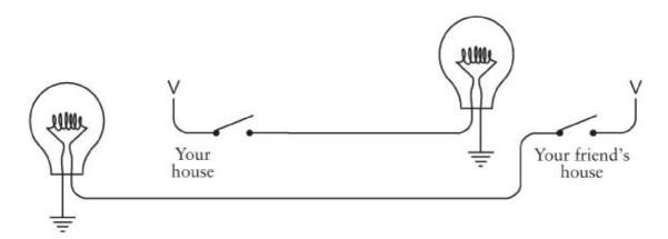
This circuit is functionally the same as the configuration shown previously, in which three wires crossed the fence between the houses.
