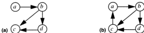
Figure 3–5 The rule of acyclic creates . (a) The can-create relation cc = \{ (a, b), (b, c), (b, d), (d, c) \} . Because there are no cycles in the graph, cc satisfies the rule of acyclic creates . (b) Same as (a), except that the can-create relation is cc' = cc \cup \{ (c, a) \} , which induces a cycle; hence, cc' does not follow the rule of acyclic creates .
