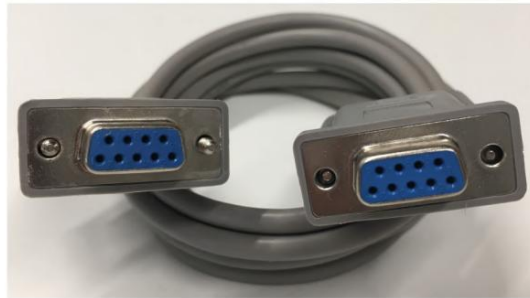
Fig. 2. A serial cable with 9-pin female connectors.
