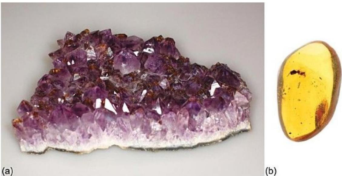
FIGURE 1.3 Examples of different solids, (a) amethyst, a crystalline solid and (b) glassy amber, an amorphous solid.
