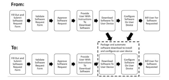
Here it has been determined that activities to download software can be automated such that the download and configuration steps can be done in a single step.
