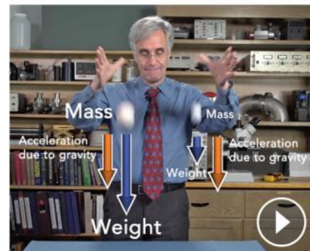
Fig. 1.2.2 A baseball (left) and a golf ball (right) both accelerate downward at the acceleration due to gravity. Their differences in weight and mass perfectly compensate for one another.
