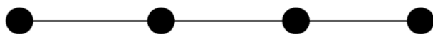
Fig. 2.5. A chain is the most fragile structure of all. The removal of any node breaks it. Thus all nodes are single points of failure.
