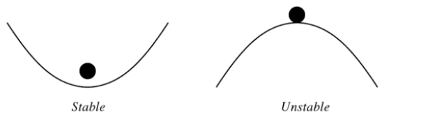
Fig. 2.1. A ball in a potential can be stable or unstable to small perturbations of ball movement. A potential well (left) is stable to movement, but unstable to filling. A potential hill (right) is unstable to movement but stable to filling.
