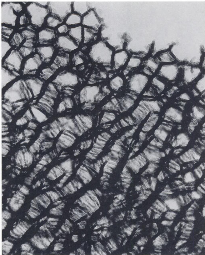
FIGURE 1.24 When etched into tiny wires no more than a few nanometers across (dark regions in this electron micrograph), silicon will emit visible light efficiently. (Photograph courtesy of Leigh Canham, Defence Research Agency, Malvern, U.K.)
