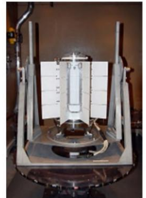
Figure 15: Nuclear thermoelectric power system for Mars rover.
