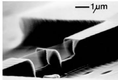
Fig. 1.22. Thinning of a GaAs mesa for TEM observation
