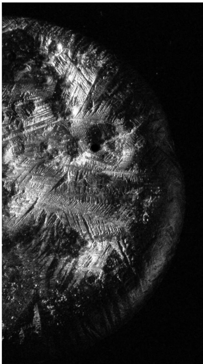
FIGURE 2.1. The star regulus of antimony, so called because of its fern- or star-like crystalline surface. The pattern is produced when the regulus of metallic antimony is allowed to cool slowly under a thick layer of the slag left after its reduction from stibnite. Prepared by William R. Newman in the laboratory of Dr. Cathrine Reck in the Indiana University Chemistry Department.
