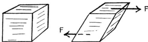
FIG. 5-7a. SHEARING. As a cubical block is sheared, its square sides become diamonds.
