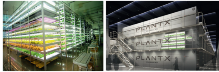
FIGURE 3.13 Left: The area ratio of total cultivation rack to floor area is about 0.5, and the area ratio of total cultivation bed area to floor area of cultivation room is about 5, in a typical conventional PFAL with 10 tiers for commercial production. Right: The area ratio of total cultivation rack to floor area is about 0.8, and the area ratio of total cultivation bed area to the floor area is nearly 10 ( = 0.8 \times 4 \times 3 = 0.96 ) in a three-stacked cultivation system modules (CSMs) each with 4 tiers with total of 12 ( = 3 \times 4 ) tiers for commercial production (to be built in 2022). The area for automatic push-in/pull-out of cultivation panels is located at right side of each CSM. The plants are harvested after transported to a separate space. Photo: by courtesy of PlantX Corp.
