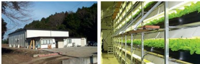
FIGURE 2.6 A PFAL with fluorescent lamps built in 2000 at Kashiwa, Chiba Prefecture, for commercial production of leafy vegetables. Courtesy of Wataru Shirao.
