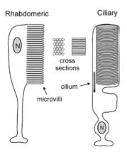
4. Rhabdomeric and ciliary photoreceptors, based on a receptor from the fruit-fly *Drosophila*, and a human rod. N is the nucleus. At the base of each receptor is the synaptic junction that connects with the nervous system
