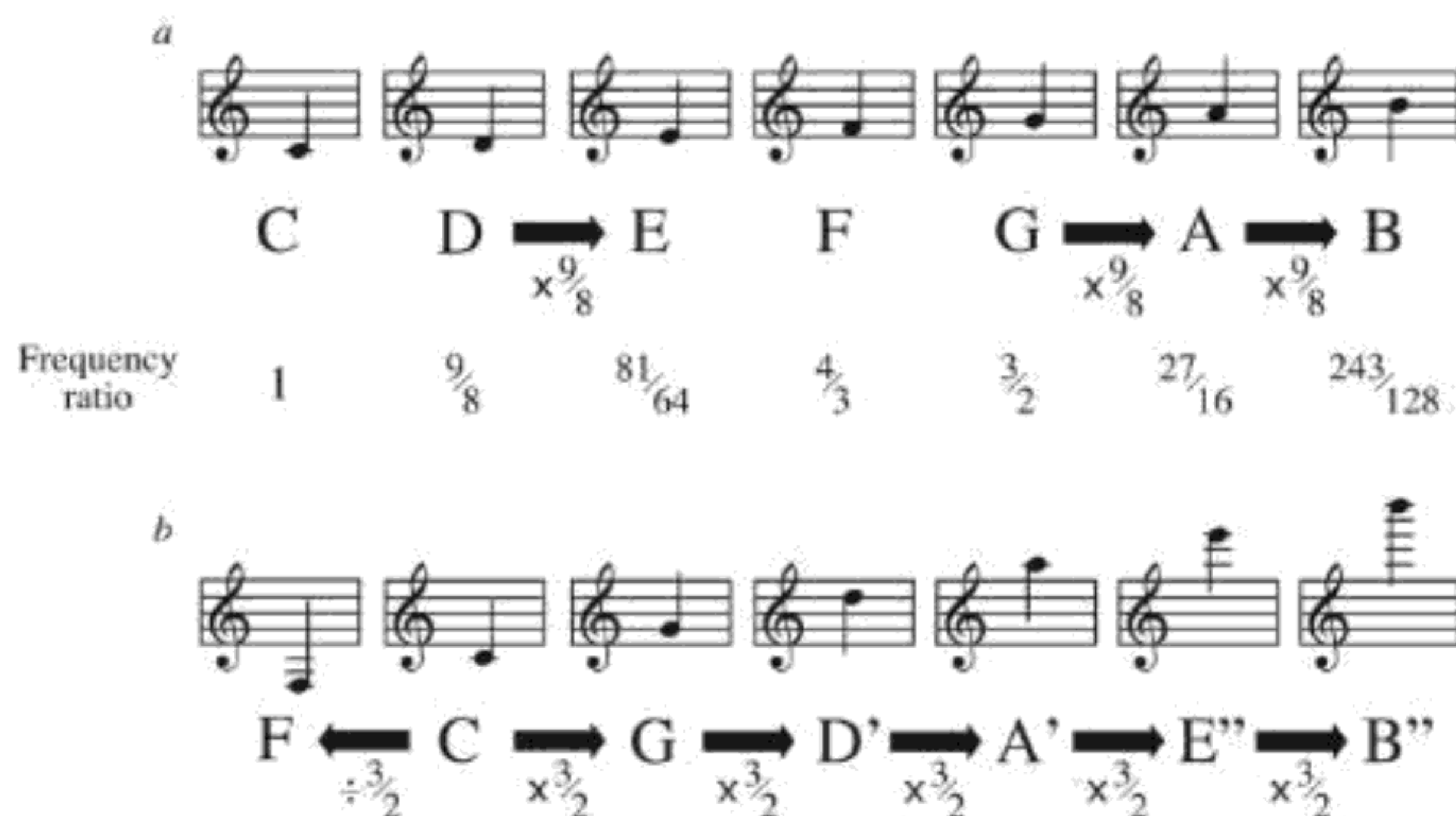
Figure 3.9 The other notes in the major scale can be 'filled in' by using the same whole-tone step of a 9/8 frequency increment ( a ). Equivalently, all the notes can be obtained through a repeated upwards step of a fifth (or downward to reach F), followed by 'folding' the notes back into a single octave span ( b ). The result is the Pythagorean tuning.
