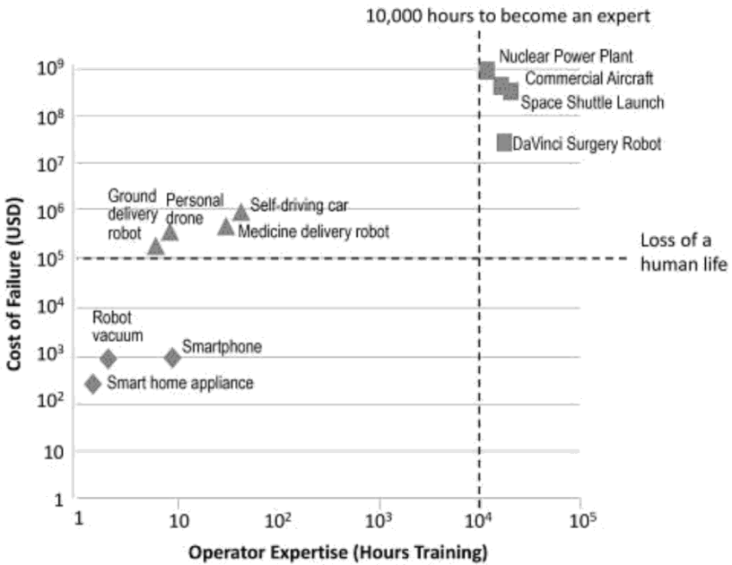
FIGURE 2: A comparison of operator expertise, measured in hours of training and cost of failures, for three classes of applications: industrial applications (squares), commercial products (diamonds), and a new class of safety-critical commercial products (triangles). Source: Laura Major and Caroline Harriott, "Autonomous Agents in the Wild: Human Interaction Challenges," in Robotics Research: The 18th International Symposium ISRR , ed. Nancy M. Amato, Greg Hager, Shawna Thomas, and Miguel Torres-Torriti, Springer Proceedings in Advanced Robotics, vol. 10 (Cham, Switzerland: Springer, 2020).
